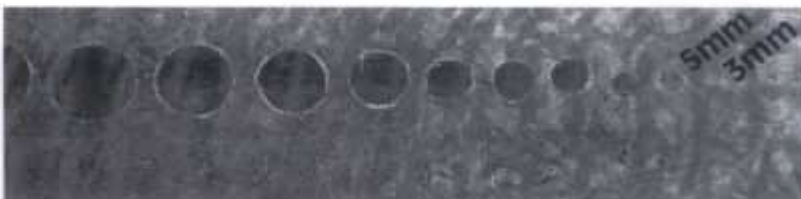
Galvanized test material that has been lost its zinc coat before it tested in industrial area, the picture show that corrosion can be prevented for diameter up to 3 mm, and minimum for dia 5 mm
