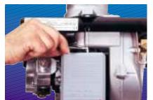
▶ The pressure regulator is carried out by setting the adjustment scrow.
