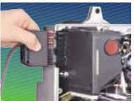
7-pole socket incorporated in the control box
