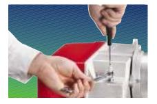
▶ 1<sup>st</sup> stage air damper position adjustment.
