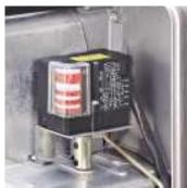
Example of air setting servomotor
