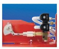
Example of air damper indexed selector and hydraulic ram of PRESS G burners
