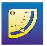
Example of fan air gate valve indexed selector of RL 28/1 burner
