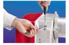
▶ 1st stage air damper position adjustment
