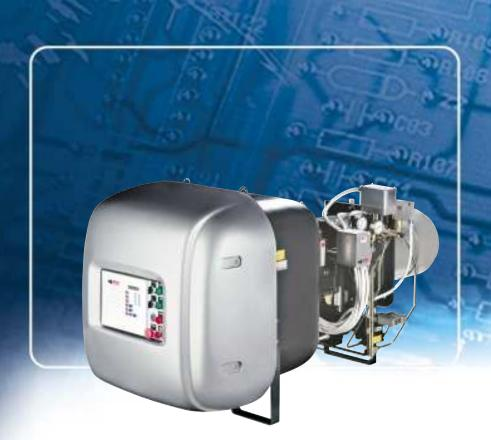
The MODUBLOC MB LE series of burners are characterised by a monoblock structure that means all necessary components can be combined in a single unit, making installation easier and faster. The series covers a firing range from 1070 to 10000 kW, and they have been designed for use in hot water boilers or industrial steam generators.
