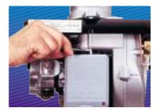
▶ Changing the position of the small plug in the economizer, the burner can remain permanently in the 1st stage, 2nd stage or works in two stage operation.
