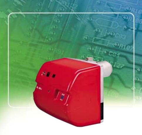
The RL BLU series of burners have been designed for use in hot or superheated water boilers, hot air or steam generators, diathermic oil boilers. The series includes two models with output ranging from 95 to 356 kW. A servomotor with three adjustable positions guarantees correct air output and air damper closing when the burner is turned off.
