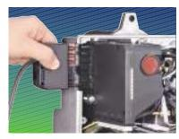
7-pole socket incorporated in the control box
