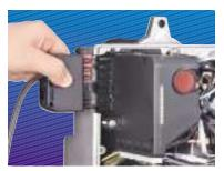
7-pole socket incorporated in the control box
